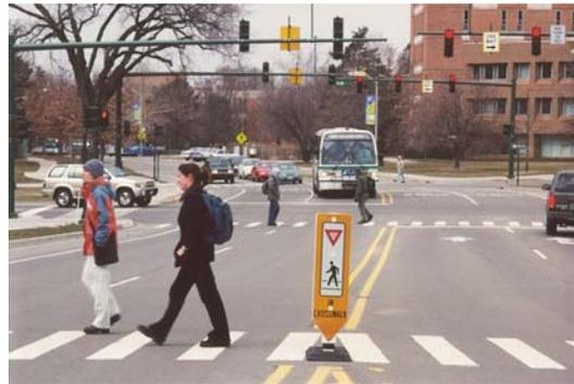
Fifteen "Yield to Pedestrian" signs mounted to RubberTough® posts from the Safe-Hit division of Quixote Transportation Safety, Chicago, Ill. were rotated around campus during the 2001 – 2002 school year. The signs were put out each day from 7 a.m. to 6 p.m. when traffic was at its heaviest.
